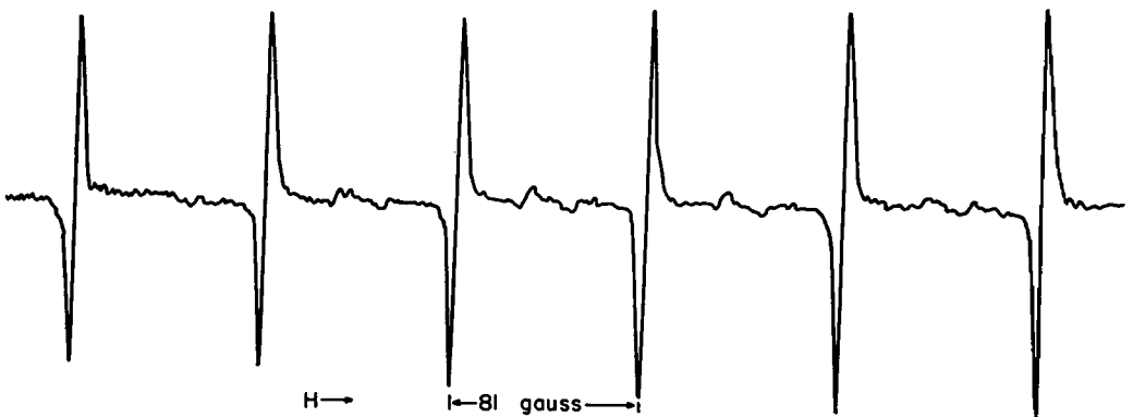
FIGURE 4 The epr spectrum of Mn^{2+} (at 200 molar ppm) in MgO .
